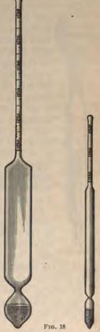
this score a sample should be analyzed. As the proper performance of a battery depends very much on the condition of the electrolyte, hydrometer readings should be taken at regular weekly intervals.
